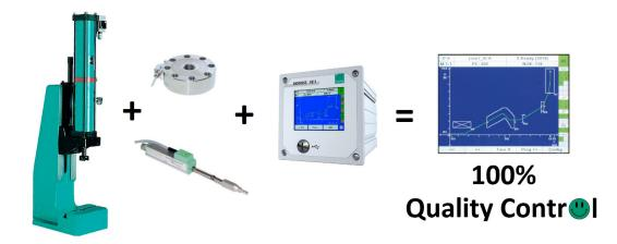
AGT offers tailored solutions aimed at monitoring the force versus displacement in pressing applications. A typical setup includes a load cell, sized for the application, and a displacement sensor to track the press operation's full travel. These sensors connect to an instrument that records measurements, plots them, and compares them to a predefined "good" signature.
