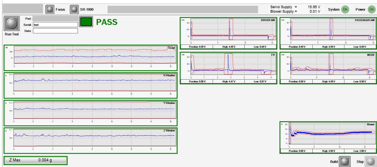
HVAC Graphical Display shown, up to 6 Servo currents, Blower current, Sound & Vibration.
