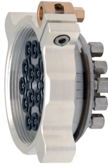
SQDC-R-16-03-P-E9-G-1 19 way removable half. Compression fittings and ferrules for 1/16 inch tubing. FFKM seals and CAM lock main nut.
