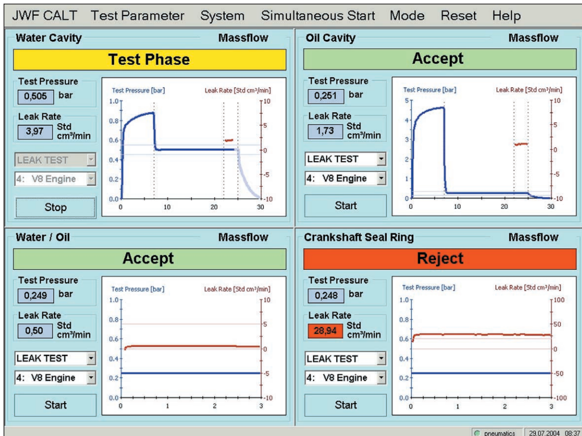
Display of a 4 Channel MFL 400 after leak testing of an engine assembly.
