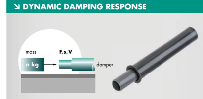
When monitoring e.g. furniture dampers, force and displacement over a defined period are measured in order to test and evaluate the damping response during the approach of an accelerated mass.
