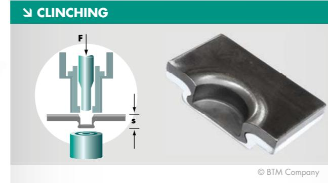
The flow process produced in the two sheet metal parts by the clinching stamp and die is monitored by a force/displacement measurement.
