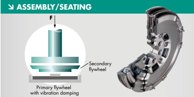
Monitoring primary and secondary flywheels of a dual mass flywheel during assembly.
