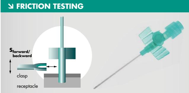
Testing the ease of movement of a venous cannula over the length of the steel insertion needle. The clasp holds the cannula and moves it up and back over the needle.
