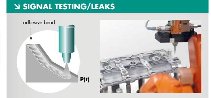
Checking for continuous application of adhesive beads, e.g. to prevent leaks from gaps in the adhesive joint. This is done by monitoring the pressure/time curve in the dispensing line.
