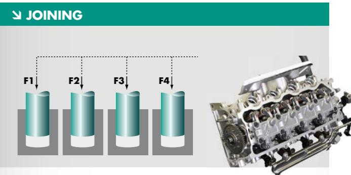
Multichannel monitoring of joining process in cylinder head assembly. The synchronous process during the assembly of valve seating rings and valve guides is measured and analyzed. DigiControl PC software logs and visualizes the process data from up to 32 controllers.
