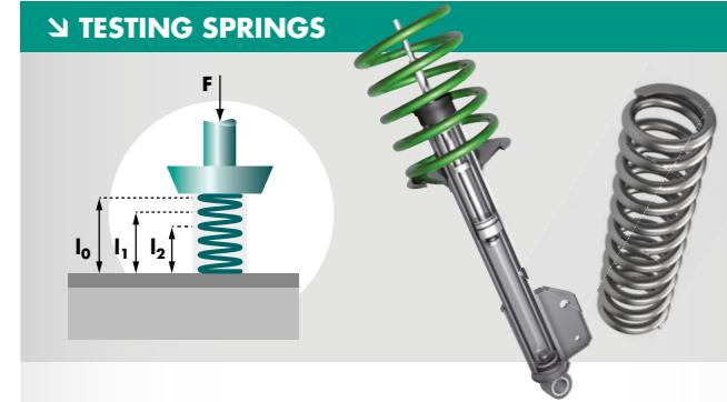
Testing of spring constant and hysteresis between applying and removing load.
