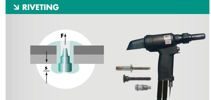
Monitoring the setting process when riveting ABS components. The oil pressure and oil volume flow rate are measured and analyzed at the hydraulic setting tool.
