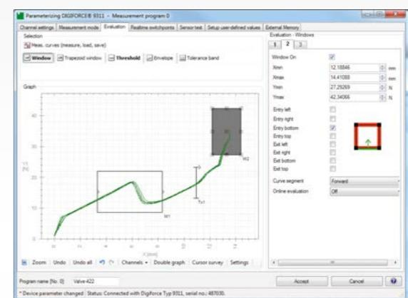
The window, trapezoid, threshold and envelope evaluation elements can be configured using the DigiControl PC software or directly from the touchscreen of DIGIFORCE® 9311.
