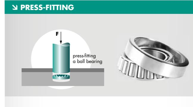
Monitoring the press-insertion of ball bearings in bearing cups.
