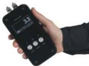
■ T2710 (with flow rates up to 0.2 l/min) and M2730 (with flow rates from 1 to 20 l/min) are the new "M series" portable digital calibrators by FORTEST. Enclosed in an anodised aluminium box provided of a shatter-proof Plexiglass front panel, we find brand-new mother board and mass flow sensor for the direct measurement of leakage. Supplied with a micrometer nozzle, it is aimed at simulating the desired leak rate, as to make the tester set up and verification easier.
