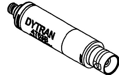
4. MATERIAL, BNC CONNECTOR: NICKEL PLATED
