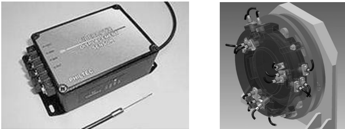
Figure 4-1 Fiber optic Displacement sensor from Philtec (left) and their installation to the measurement setup (right)
