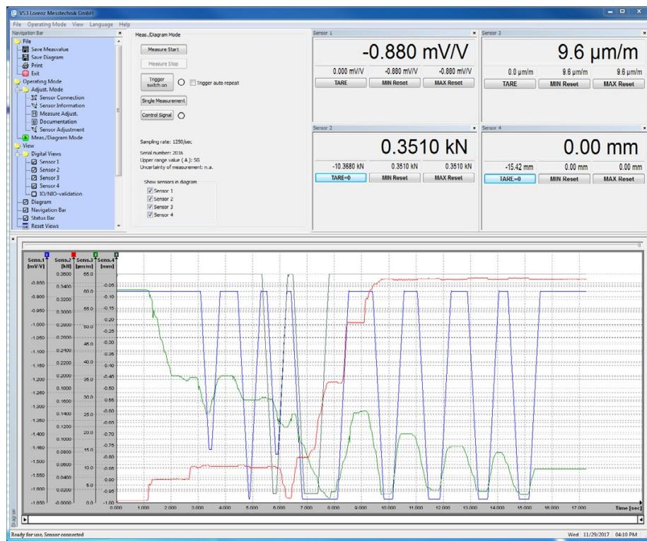
The configuration and evaluation software serves for easy evaluation and graphical visualisation of the evaluated data on a PC.
