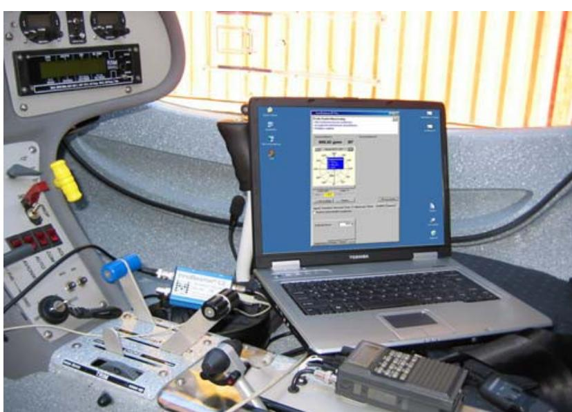
The user is guided through the balancing process by VM-BAL software. The system detects the unbalance and informs about necessary compensation measures. The optimum compensation method can be chosen according to the application. Fixed angle positions at the rotor can be calculated for attaching or removing weight using various methods. Thanks to the automatic rotation speed detection, the hands are free during the measurement.
