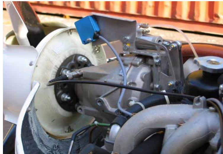
Metra's **VMBAL Kit One** is employed, a complete solution for Single-Plane-Balancing with all necessary sensors, measurement equipment and PC-software. Dynamic balancing offers an efficient way to balancing success based upon measurement results and calculations. The user does not need to take care of these calculations.
