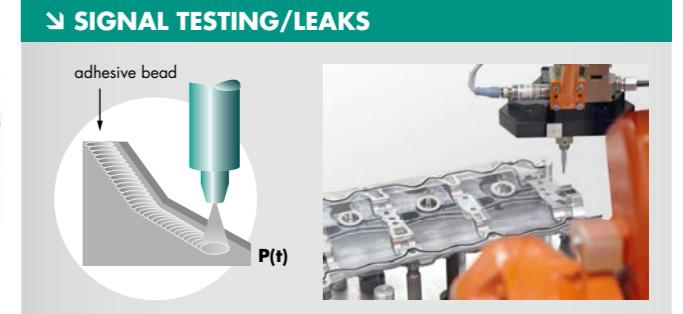
Checking for continuous application of adhesive beads, e.g. to prevent leaks from gaps in the adhesive joint. This is done by monitoring the pressure/time curve in the dispensing line.
