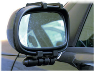
D x mirror antenna for unobtrusive placement during road tests
