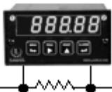
**External current shunts are fully supported.** Scaling from full-scale millivolts, such as 50 mV or 100 mV, to amperes is easily accomplished from the front panel of the meter. The scalable display is five full digits up to  $\pm 99,999$  counts.
