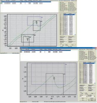
Display of the force displacement diagram and switch point with magnifier function truments <u>Ltd.</u>
