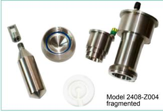
Measurement cell model 2408-Z004 with Guard-ring for measuring of the resistance  $R_{\scriptscriptstyle D}$  and specific resistance  $\rho_{_D}$  (resistivity) of electrical insulating liquids regarding IEC publ. 247, DIN 53482 / VDE 0303.
