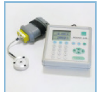
Force calibration using the DIGISTANT®, Smart Sensor Interface and force sensor
