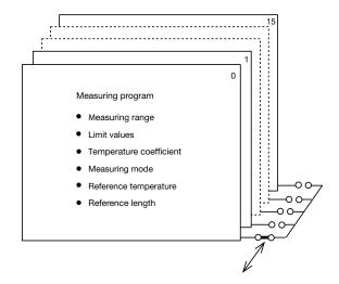
For fast object changes, RESISTOMAT® 2316 can store up to 16 measurement programs, which can be executed either by PLC, by hand or RS232 (USB, Ethernet)
