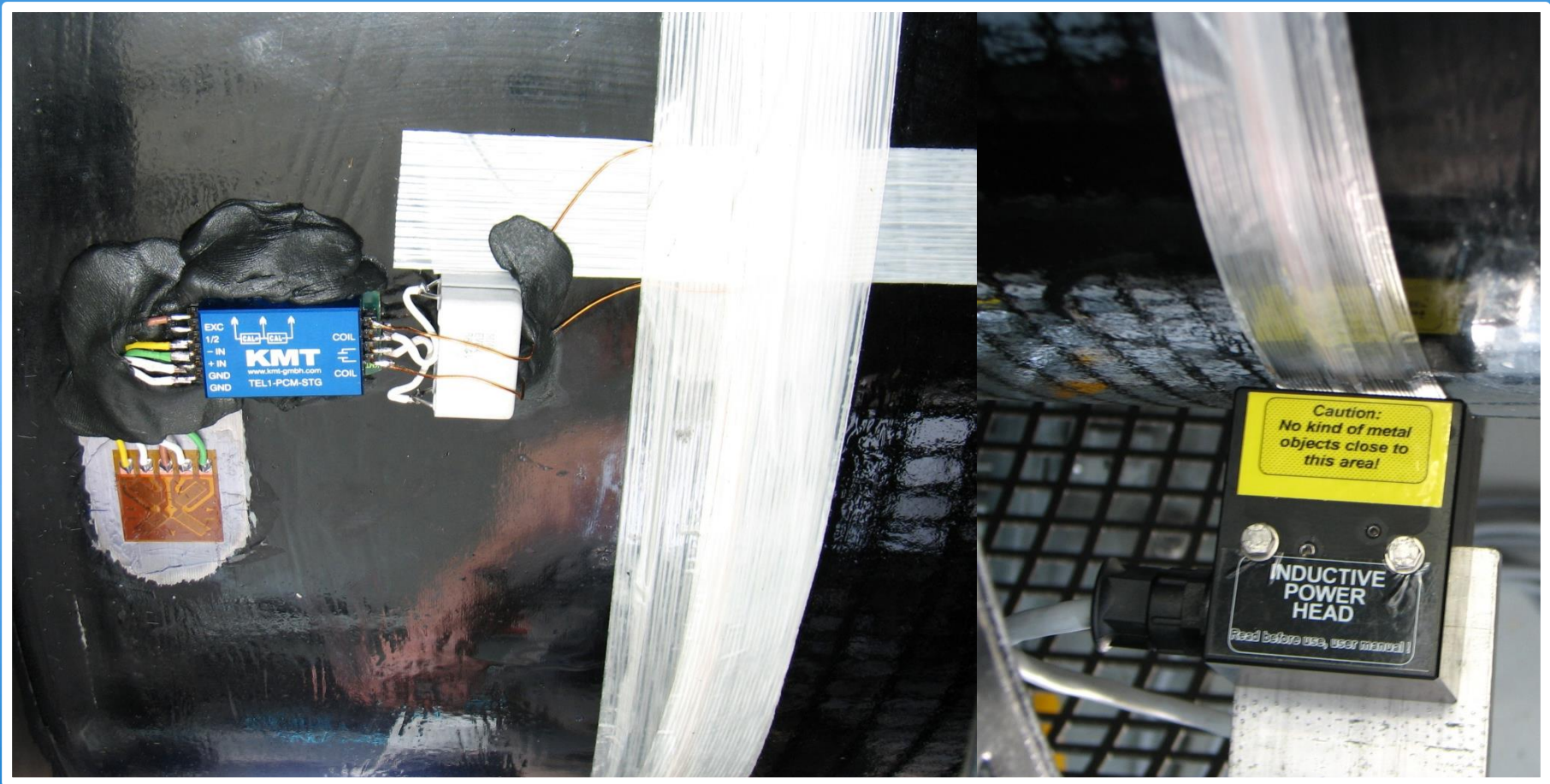
TEL1-PCM – Torque Telemetry “torque measurement on low-speed shaft”
