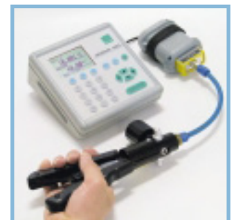
Pressure generation with hand pump
