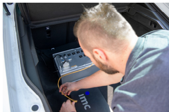
Fig. 2: Connecting to CAN bus and Wi-Fi
