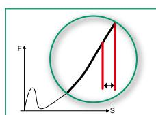
This option is used for monitoring deformation of the workpiece around the maximum force. This is done by measuring the displacement when the force exceeds the "lower block limit".
