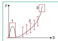
Within this area, the measurement process can be monitored for exceeding a maximum force (upper feed-in limit). Good parts are not allowed to exceed this limit.
