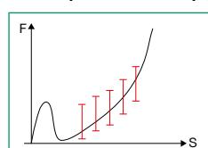
With force-displacement limits, the force in this area must always exceed a minimum force (lower force limit). The force must then not drop below this limit again over the entire area. For good parts, the force must also not exceed a second force limit, the "upper force limit".
