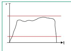
Force thresholds can be used to monitor whether the force lies in a defined range. A green light indicates that the force lies in the specified range. A force that exceeds the upper force threshold triggers a visual and acoustic alarm. Evaluation takes place online during measurement.
