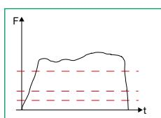
In addition, 3 limits are available for defining various switching results. With hysteresis settings, a limit buffer and customizable switching behaviour, these switching results can be tailored to customers' requirements. There is also a facility to delete the limit via a digital input.
