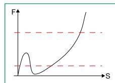
In addition to the evaluation areas ① - ③ force alarms 1 and 2 are always available. Force alarm 1 is used to monitor the load cell outside a started measurement. Since this is monitored over the displacement, this force monitoring is not enabled for the  $Y=f(t)$  function (no displacement measurement).
