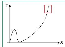
This area is usually where the end of the measurement lies, which a good part must always reach. The force limits "lower block limit" (which must be exceeded) and "upper block limit" (which the force must not drop below) are used to monitor the block force.
