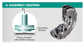
Monitoring primary and secondary flywheels of a dual mass flywheel during assembly.
