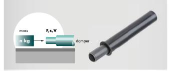
When monitoring e.g. furniture dampers, force and displacement over a defined period are measured in order to test and evaluate the damping response during the approach of an accelerated mass.
