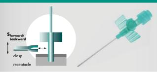
Testing the ease of movement of a venous canula over the length of the steel insertion needle. The clasp holds the canula and moves it up and back over the needle.
