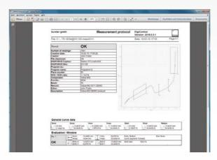
A Data-log wizard provides filters for selecting and displaying stored measurement logs. A report printout containing component data, curve information and all evaluation results can be generated for each individual measurement log.
