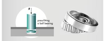
Monitoring the press-insertion of ball bearings in bearing cups.
