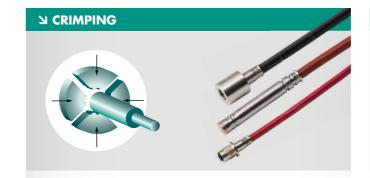
To monitor crimping processes, the force applied by the jaw segments to the material deformation is analyzed as a force/time curve. Wear to a jaw segment or breakage can be detected.
