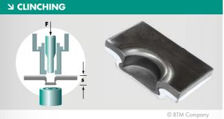
The flow process produced in the two sheet metal parts by the clinching stamp and die is monitored by a force/displacement measurement
