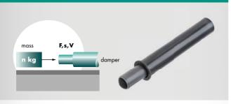
When monitoring e.g. furniture dampers, force and displacement over a defined period are measured in order to test and evaluate the damping response during the approach of an accelerated mass.
